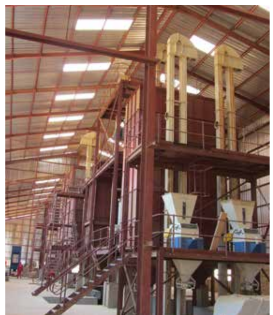
The feedmill can process 40 t/hr – one of the largest in East Africa.
